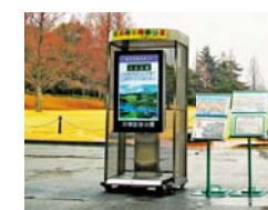
The housing is designed to cover the entire display unit to prevent injury by bumping into the display corners.
