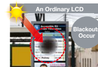
Direct sunlight raises the LCD panel temperature and causes blackouts.
